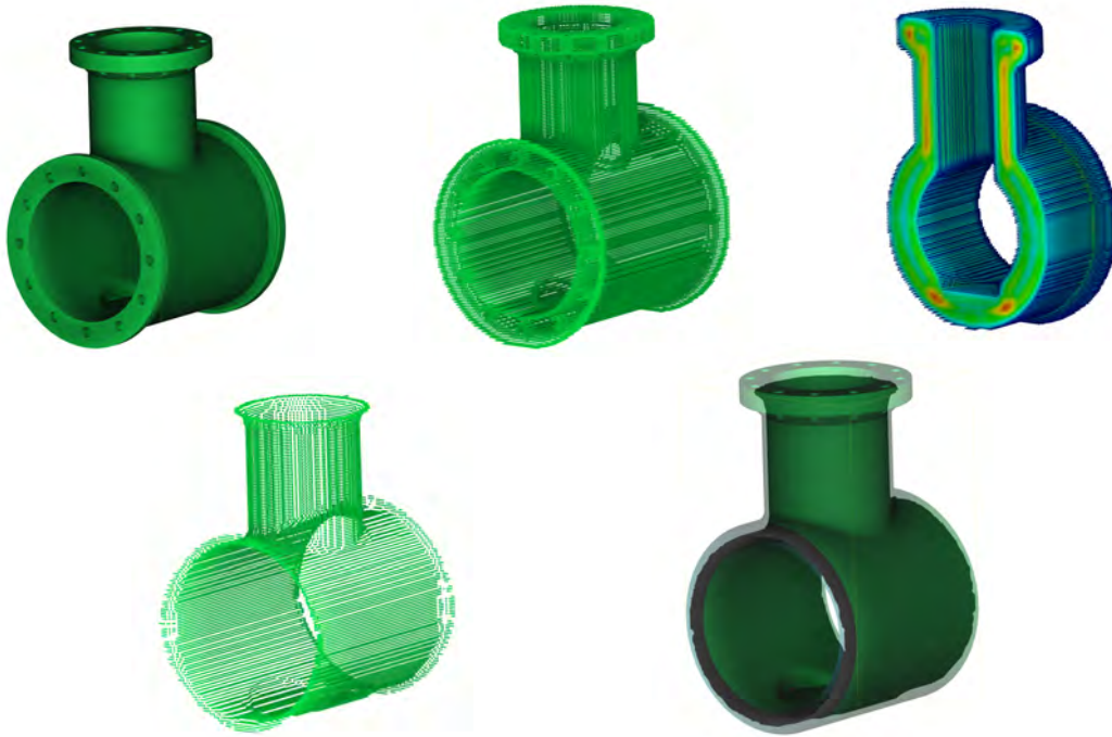
Figure 1: The new midsurface generation algorithm samples the input geometry (top row, left) to a binary 3D grid (top row, middle). Then the binary grid is interpreted as a density field and applies a kernel to it (top row, right; cut for visibility). Afterwards, the vertices of the original input data are moved within the density field towards the climax (bottom row, left). Finally, vertices which approach each other are clustered and merged. The result is a midsurface. Input and output geometry are shown in the bottom-right rendering (cut for visibility).
