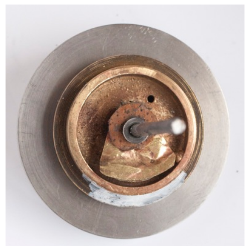
Figure 4. Wide contact covers two outlets.
