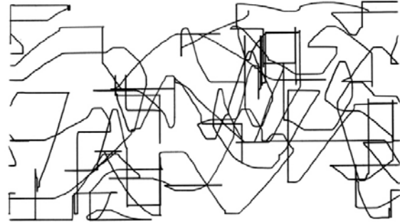
Figures 9 & 10 Flat-bed X:Y plotter drawings; presence of circles and diagonal lines show difference to New Drum images.
